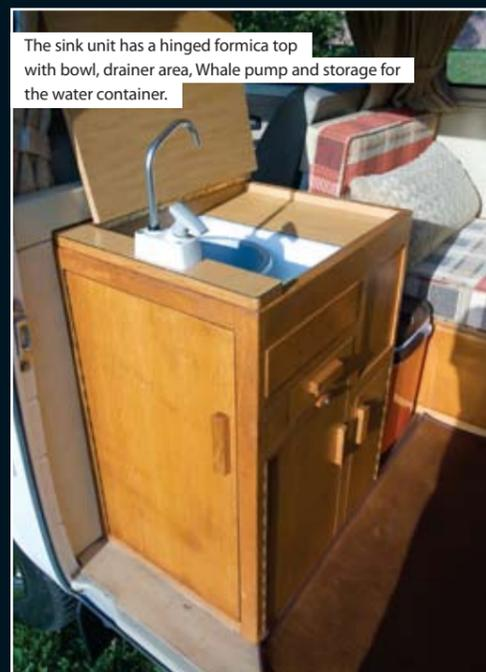
The sink unit has a hinged formica top with bowl, drainer area, Whale pump and storage for the water container.
